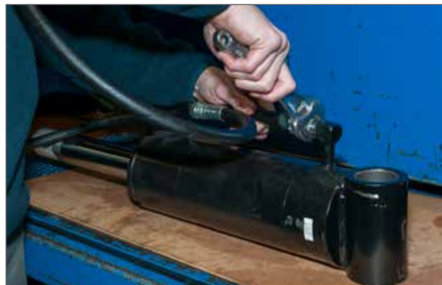
Fitting the cylinder on the test bench – adjustable height Every cylinder is tested before leaving our workshop.
