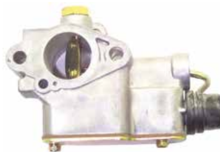
REF 107TA1854 Used for NISSAN, FHG20, 25, 30N TCM with Z24 engine
