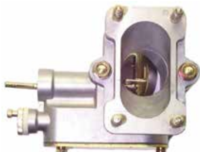
Model S276 REF 107TA1859 Used for TCM with H20 engine NISSAN
