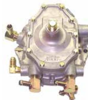
REF 107TA9360 Vaporizer used for NISSAN J02
