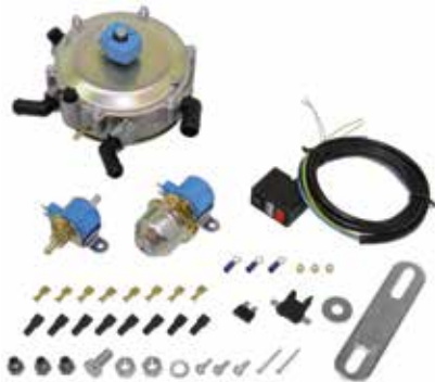
REF 143TA7622 Minikit carburettor GV090 with CL1 fuel switch
